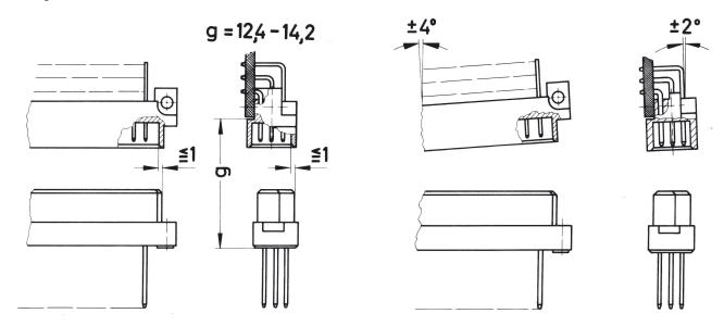
To ensure reliable connections and prevent unnecessary damage, please refer to the application data diagrams. These recommendations are set out in IEC 60603-2.
